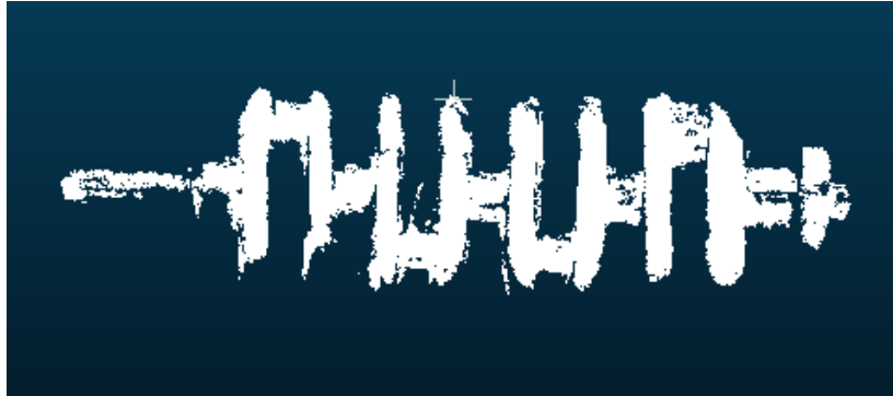
Figure 2. Point cloud from worn crankshaft
