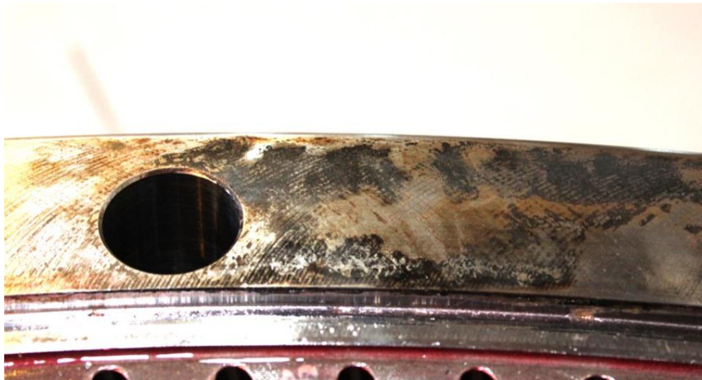
Figure 1. Example of fretting damage in bolted connection after part disassembly from field
