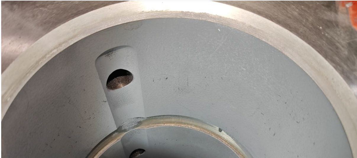
Figure 1. Enhanced coating solution testing for increased robustness in wind turbine journal bearings
