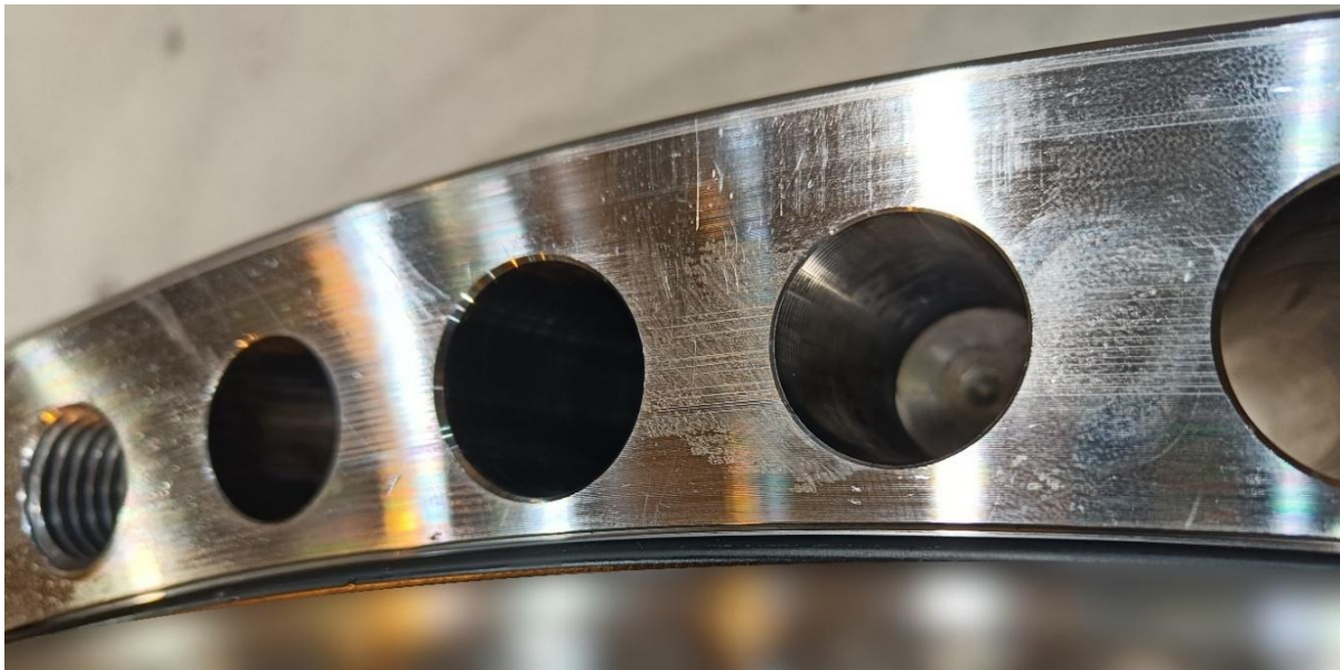
Figure 1. Fretting damage on ring gear connection after initial test without friction improvement.
