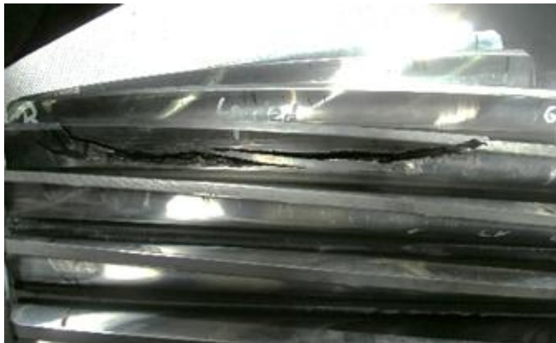
Figure 1: TFF failed tooth from a wind turbine gear in an overload test. Sudden single tooth breakage can happen after few thousand operative hours despite design lifetime being over 175 000h leading it to be considered as a premature failure. Root cause in this case was identified as subsurface inclusion bigger than allowed in material specification. [Flender Finland]
