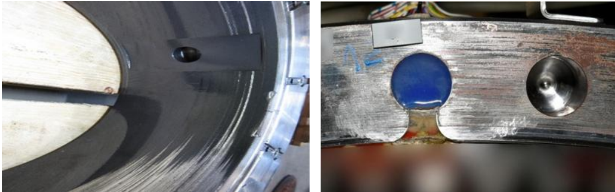
Figure 3: Left side asperity contacts and wear at journal bearing at testing component. Right side flange connection with initial fretting and wear from gear box level overload testing. [Flender Finland]
