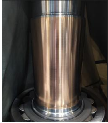
Figure 5: Laser clad journal bearing and variation between different alternatives.
